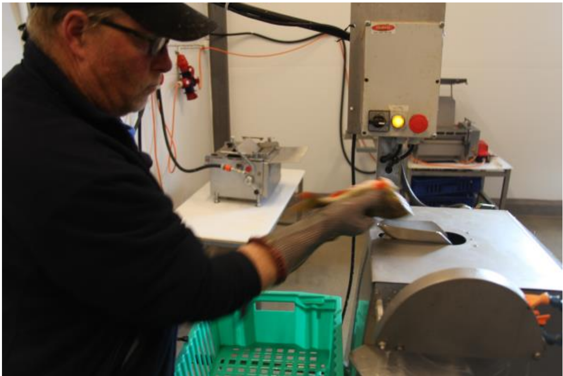
The fish is fed into the opening. The machine will split the fish and take out the bone.
