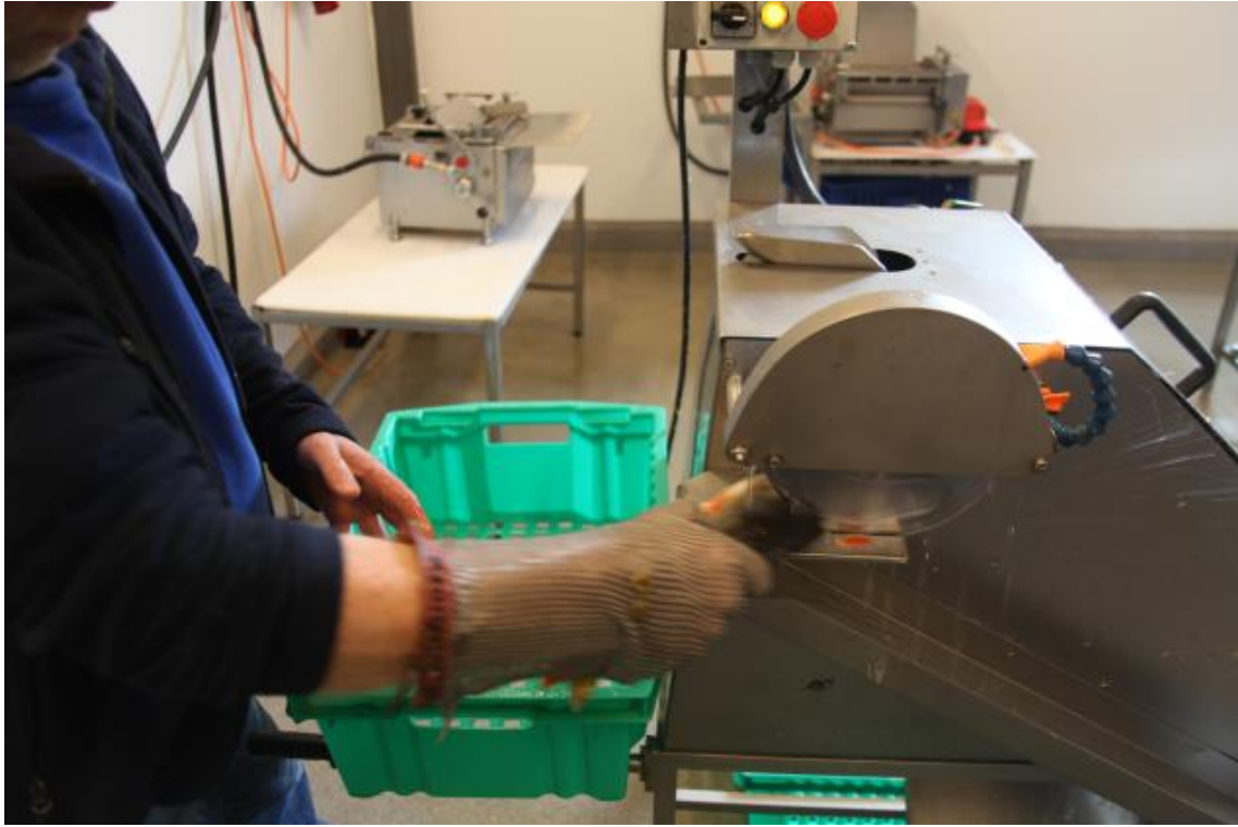
The head is first cut off with a saw at the side of the splitting machine.
