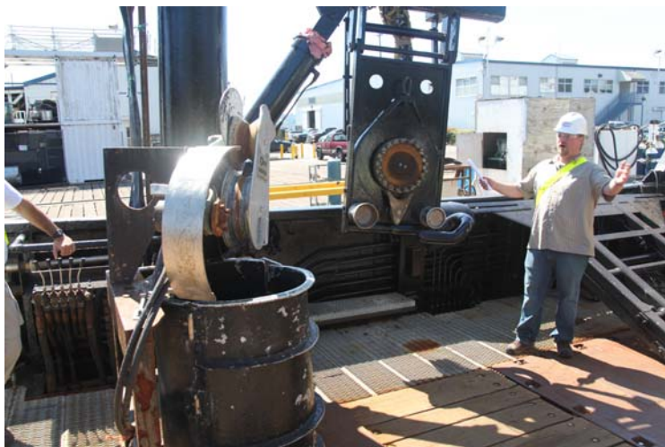
Picture 3. Demonstration of area on Trident Seafoods vessel where the crab or cod cages are lifted into the vessel and emptied into the processing line inside the vessel.
